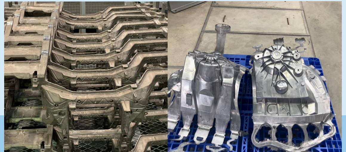
First test run successfully completed in September 2021 (Left: Cross Car Beam | Right: Shock tower)
