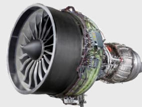
CMC is 2/3 lighter with 20% higher temperature resistance
