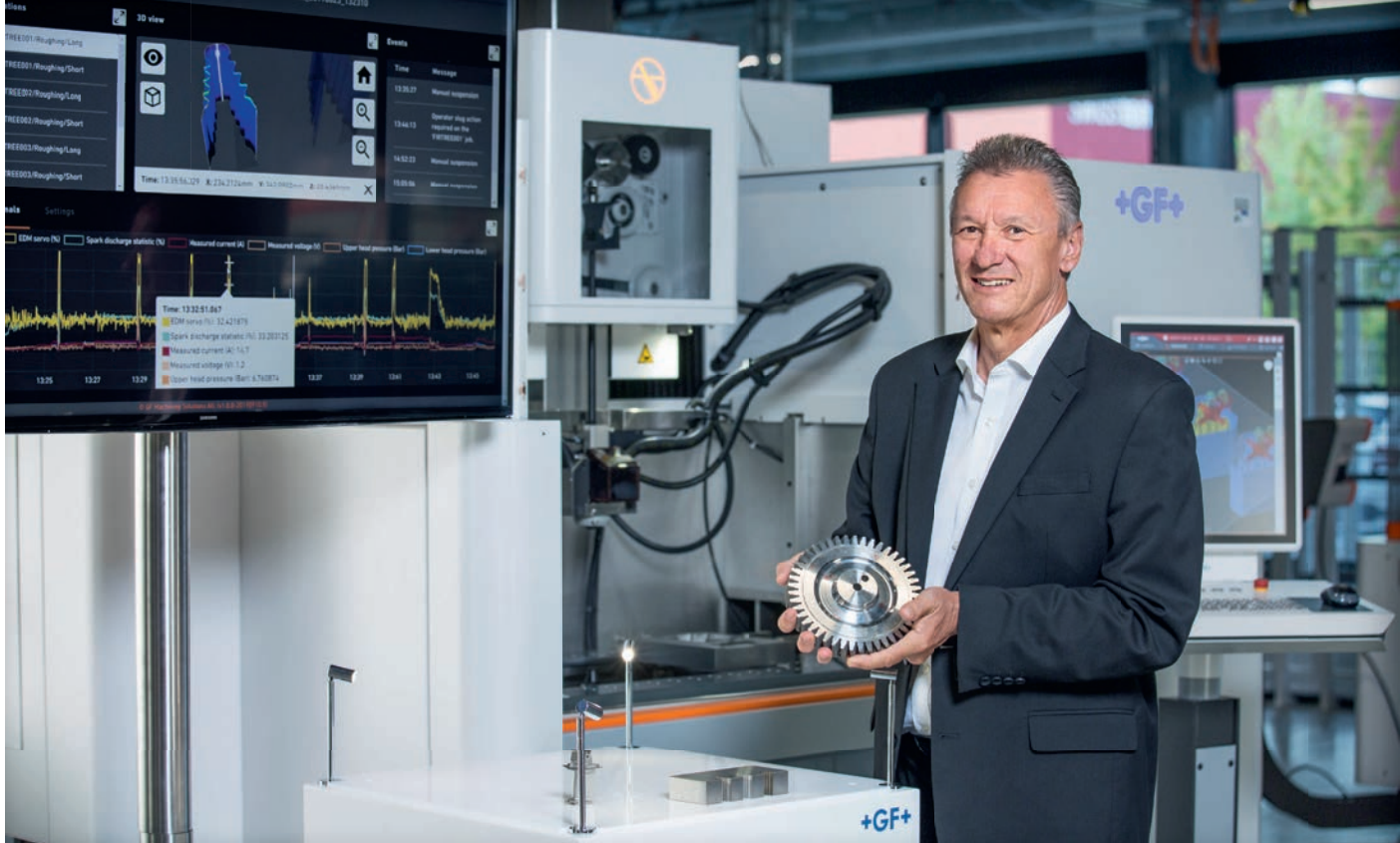
Pascal Boillat, President of GF Machining Solutions, explained at GF's Capital Market Day how a Fir Tree Disk, a part of an aerospace turbine, can be manufactured even more precisely with a Spark Track technology.
